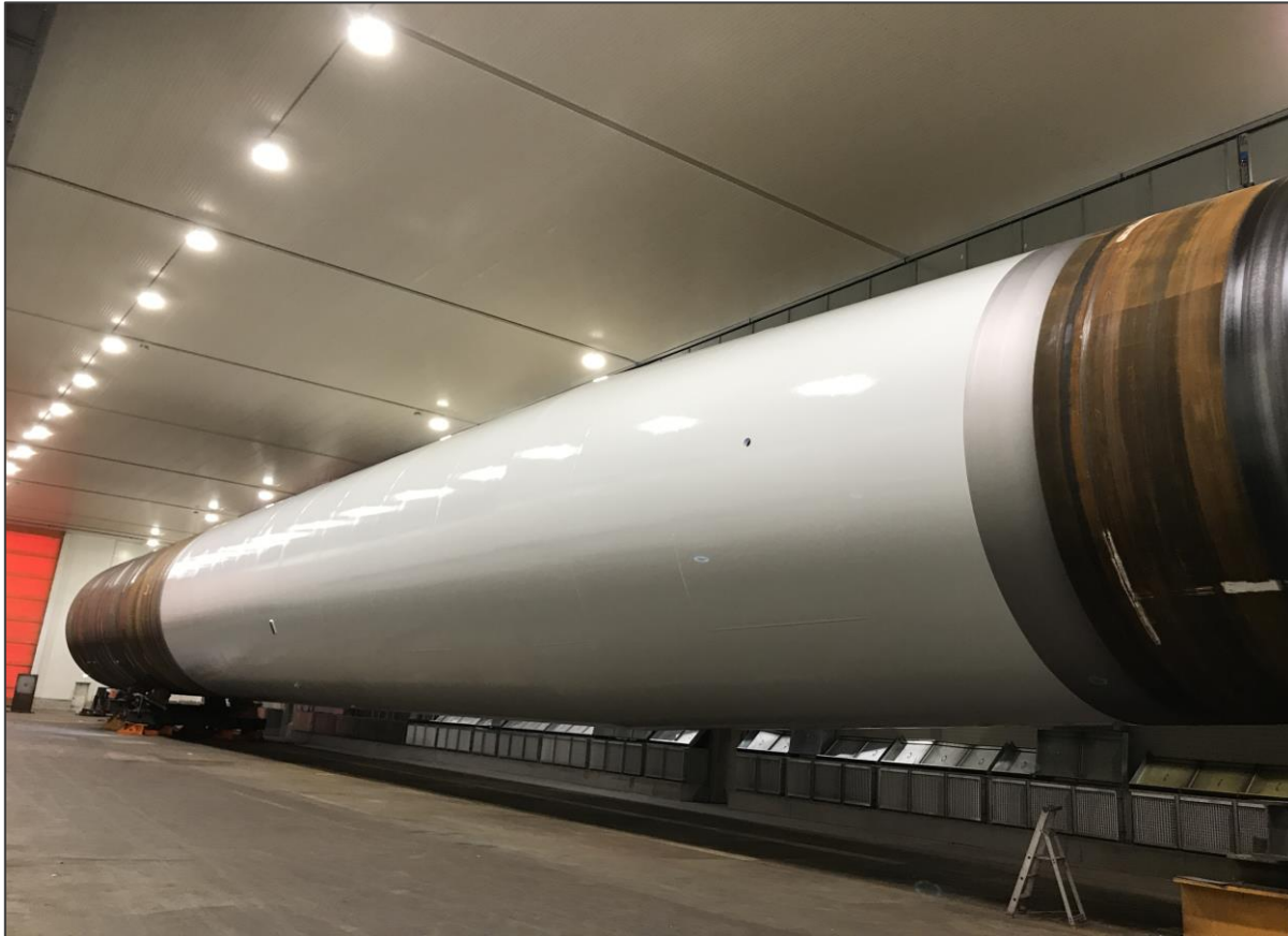
1 st coated monopile (Rotterdam, The Netherlands)
