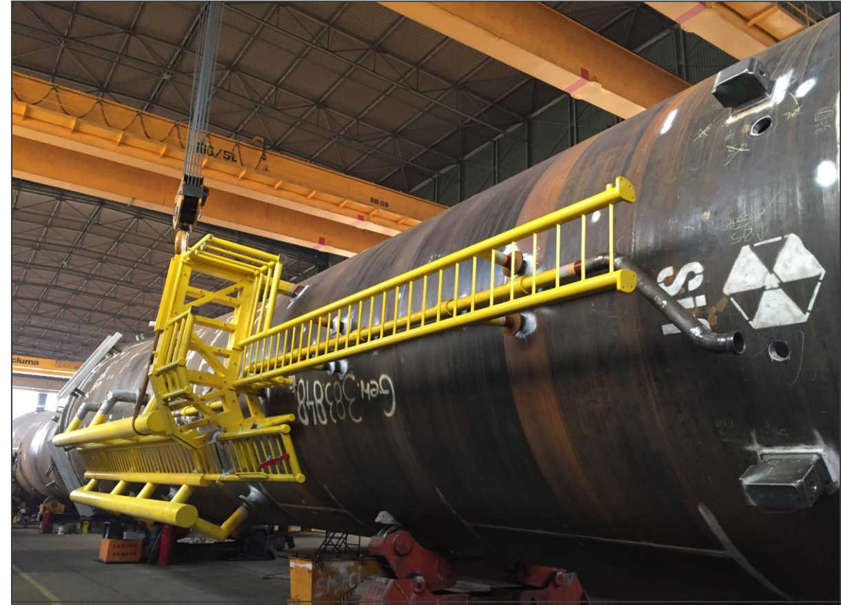
Transition piece (Hoboken, Belgium)
